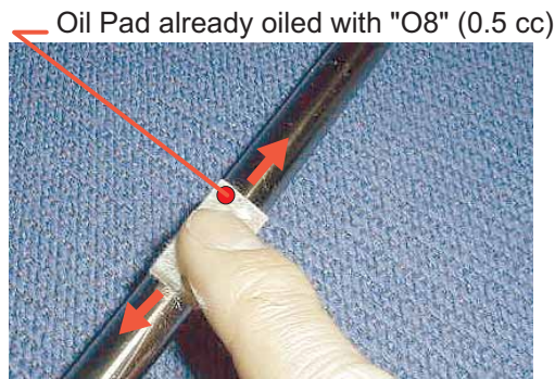
Figure 6-6. Preliminary Lubrication with "O8"
