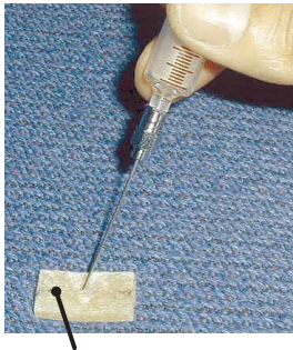
Supply "O8" (0.5 cc) to the oil pad.
